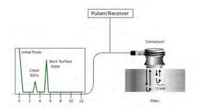
The reflected wave signal is transformed into an electrical signal by the transducer and is displayed on a screen. In the applet below, the reflected signal strength is displayed versus the time from signal generation to when a echo was received. Signal travel time can be directly related to the distance that the signal traveled. From the signal, information about the reflector location, size, orientation and other features can sometimes be gained.
