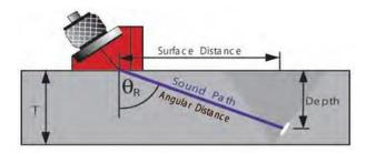
$\begin{array}{l} \theta_{\text{R}} = \text{ Angle of Refraction} \\ \text{T} = \text{ Material Thickness} \\ \text{Surface Distance} = \text{Sin} \theta_{\text{R}} \text{x Sound Path} \\ \text{Depth (1st Leg)} = \text{Cos} \theta_{\text{R}} \text{x Sound Path} \end{array}$
